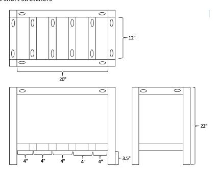
Connect with pocket hole screws. Most pocket holes on this project are on the bottom of the boards, so that they are not visible. Connect the paver to the wood base with liquid nails.
