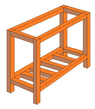
Wood Base: Overall dimensions H=22" x D=23" x W=15" Stone top (Antique Parma Travertine Paver): 16" x 24"
