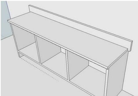
Top. Now add the second 1x12 @ 48" on top of the previous one (from step 2), placing a 1x4 behind it. Overhand the 1x4 3/4" on either end, and nail the 1x4 into the top 1x12, and the top 1x12 into the bottom 1x12. The top 1x12 should be flush on the sides, and overhand the front 3/4".
