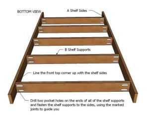
Line the top corner up with front edge of legs 33' 2" screws and glue
