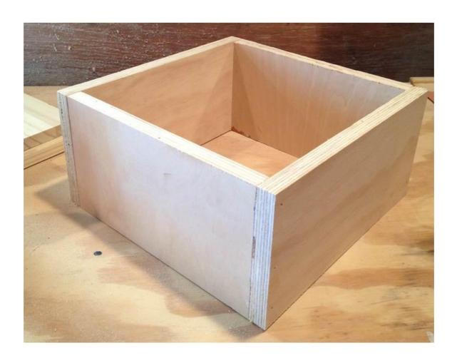
Step 2: Attach bottom to box, keeping outside edges flush. Use glue and  $1\frac{1}{4}$ " finish nails.
