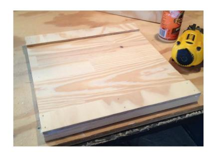
**Step 8:** Attach side trim to box top, keeping outside edges flush. Use glue and 5/8" brad nails.
