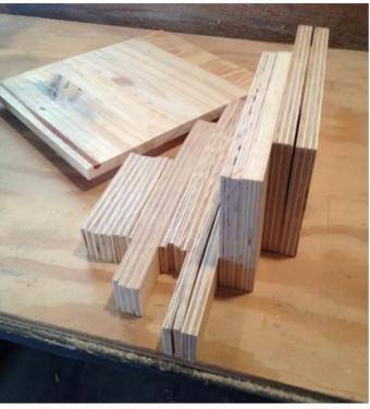
Step 1: Attach sides between front and back as shown. Use glue and 1 ¼" finish nails.
