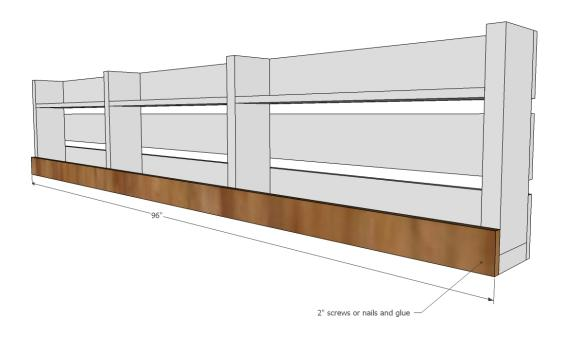
Step 4: Attach remaining front 1x4 to front with 2" screws and glue. Screws are recommended because the hooks will hold weight, pulling on this board.
