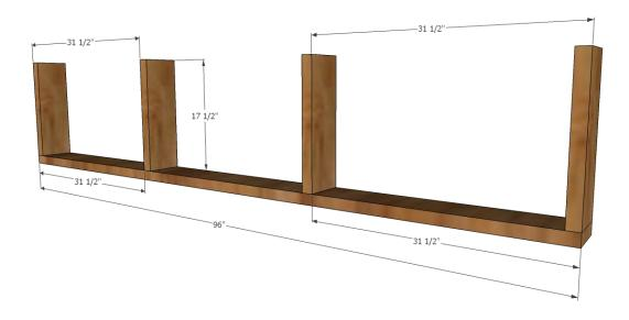
Step 1: Build the frame with the 2x6 boards. Start by attaching the outer 2x6s together, then add the center two dividers. Use 2-1/2" screws and glue.
