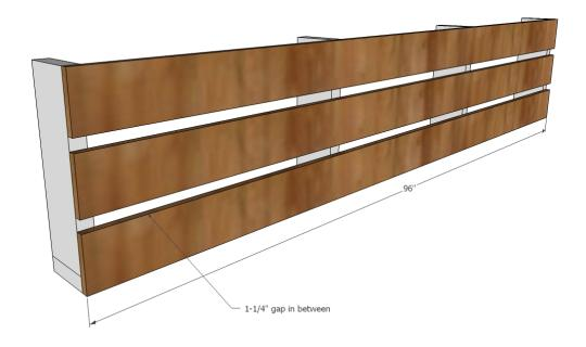
Step 3: Complete the back by attaching 1x6 boards to back with 2" screws and glue. Screws are recommended because these boards will be used for hanging the rack. Attach top and bottom first, then center middle 1x6 and attach.
