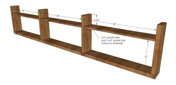
Step 2: Attach shelves using 3/4" pocket holes and 1-1/4" pocket hole screws and glue.
