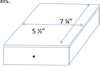
10. Attach door front to top & bottom (2 doors). 1x3 goes at the top and 1x2 goes at the bottom. The 1x2 should be flush with one side, as shown in diagram.
