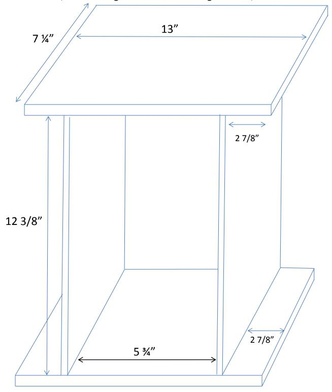
4. Attach shelves to sides, using 1 7/8" spacer to make sure shelves are spaced the same in between all the way up. Start at the bottom and repeat for each shelf. Use glue & 1 1/4" finish nails.
