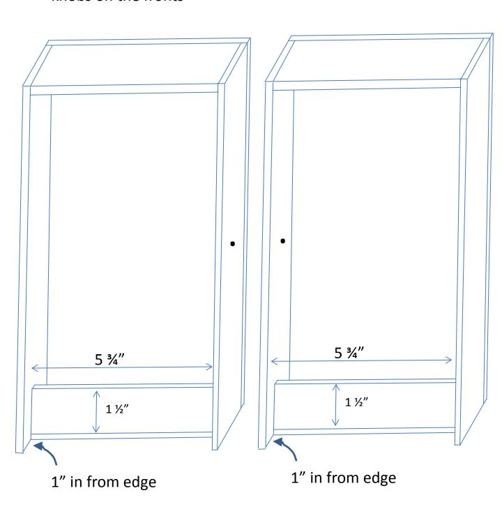
15. Attach piece of 1/2" trim to inside top of doors as shown. Glue and clamp this piece in place.
