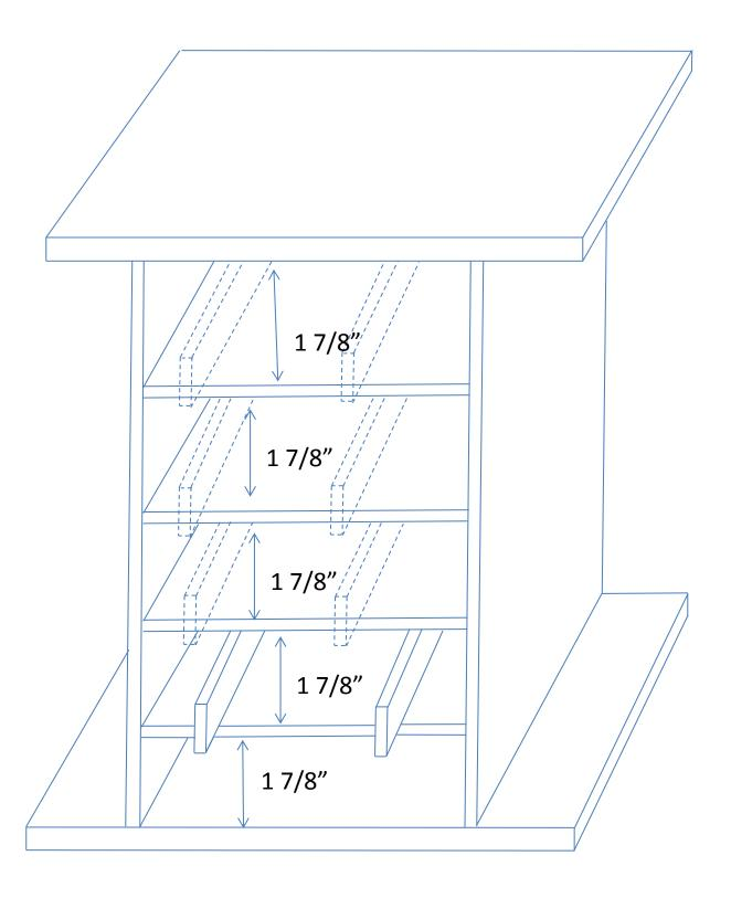
5. Attach back to box. Back only covers shelves and sides, not the overhangs. Use glue and 1" finish nails.
