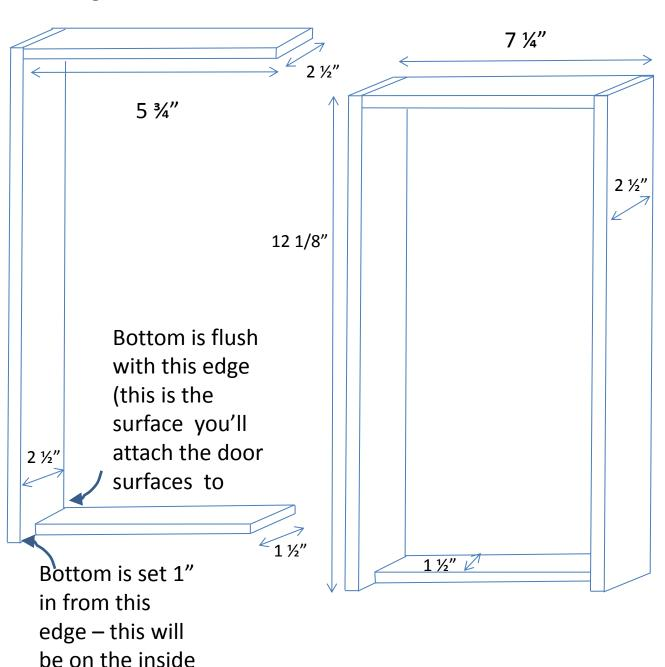
12. Attach door surface to door frame (2 doors) Use glue & 1" finish nails.
